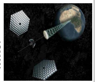
Wireless power transmission satellites are powered via PV arrays which receive solar radiation from both the sun and from the solar reflector satellites. A microwave emitter is then used to beam down energy to the habitat. Rectennas will be present on the lunar surface to harness the microwaves and convert them into DC electricity which can then be distributed either to the habitat or to the energy storage systems.
