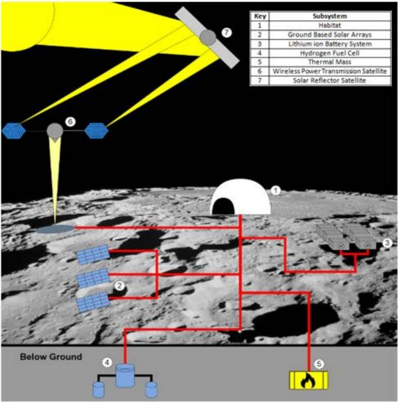
As shown, the designed power system represents a micro grid with numerous energy storage and generation options spread across the lunar surface. The satellites will be constellations to allow for constant coverage supply and to the habitat even during the lunar night.
