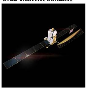
Solar reflector satellites are used to reflect solar radiation onto the PV panels present on the WPT satellites. These reflector satellites will operate using mirrors and track both the position of the sun and the position of the WPT satellite it is beaming too. A constellation of satellites is implemented to allow for constant reflecting of solar radiation to the WPT satellite even during lunar night.
