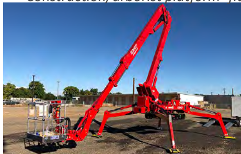
Construction/arborist platform- fits on sidewalk, 60' reach
