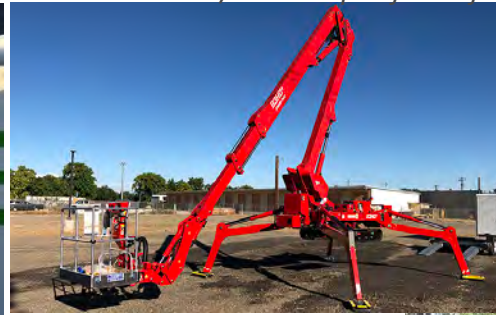
Construction/arbormist platform- fits on sidewalk, 60' reach
